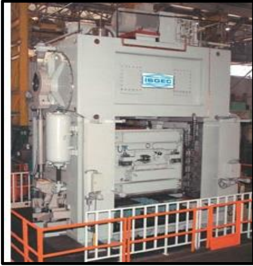
POWER PRESS 630 MTON ISGEC MAKE INSTALLED AND COMMISSIONED
