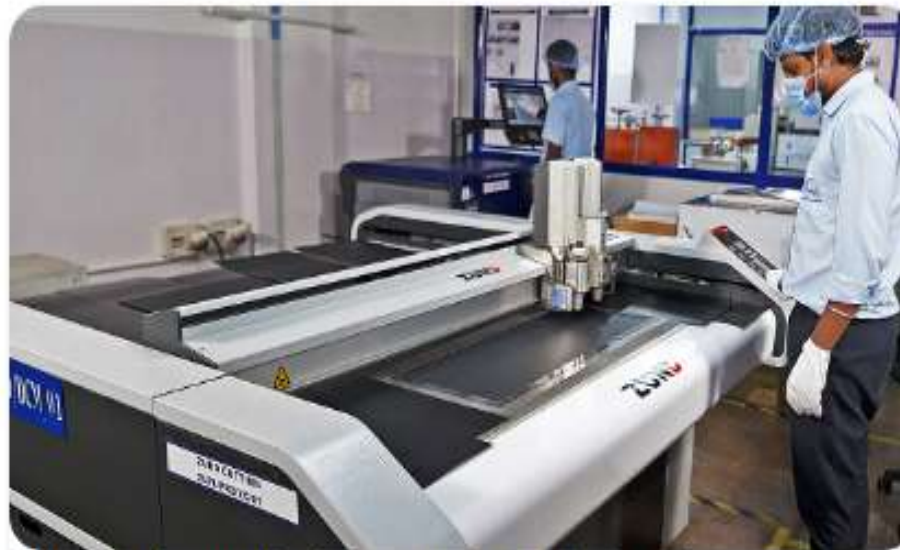
Flatbed cutting machine for custom-shaped labels and parts
