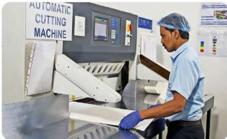
Automatic cutting machine for high-volume label production
