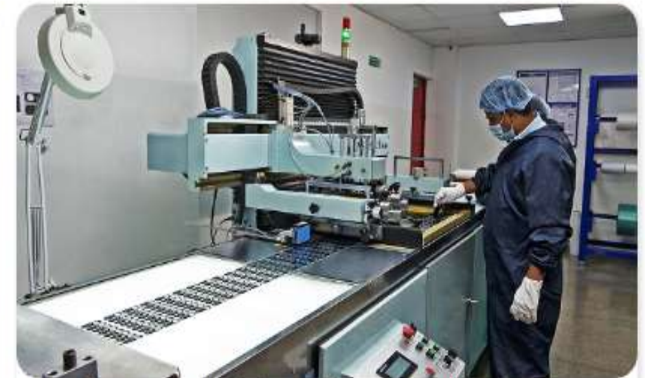
Industrial screen printing line for graphic overlays and labels
