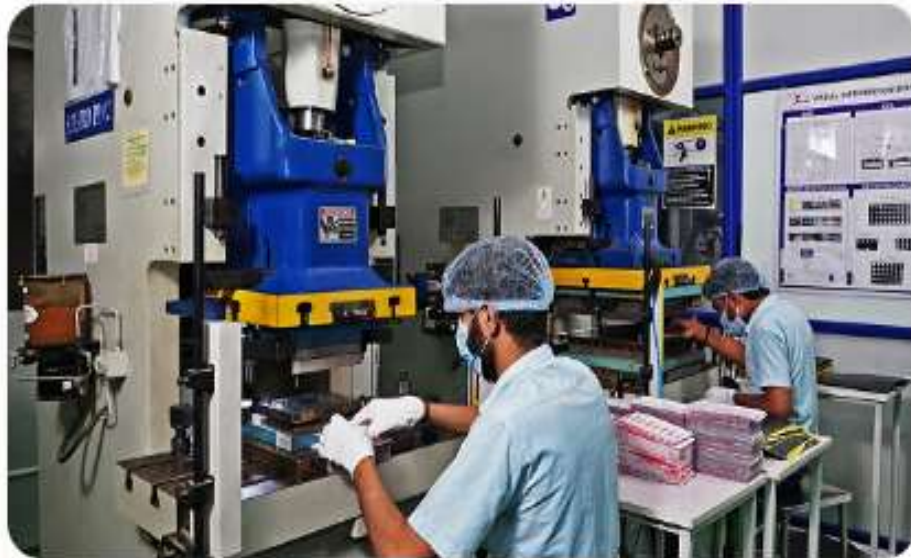
Power press machines for forming and component processing
