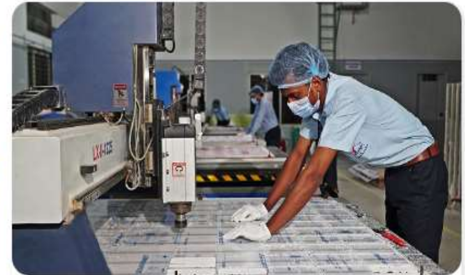
CNC routing and engraving for industrial nameplates and panels
