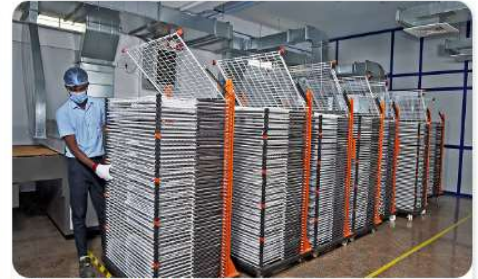
Batch-wise material handling and in-process storage system
