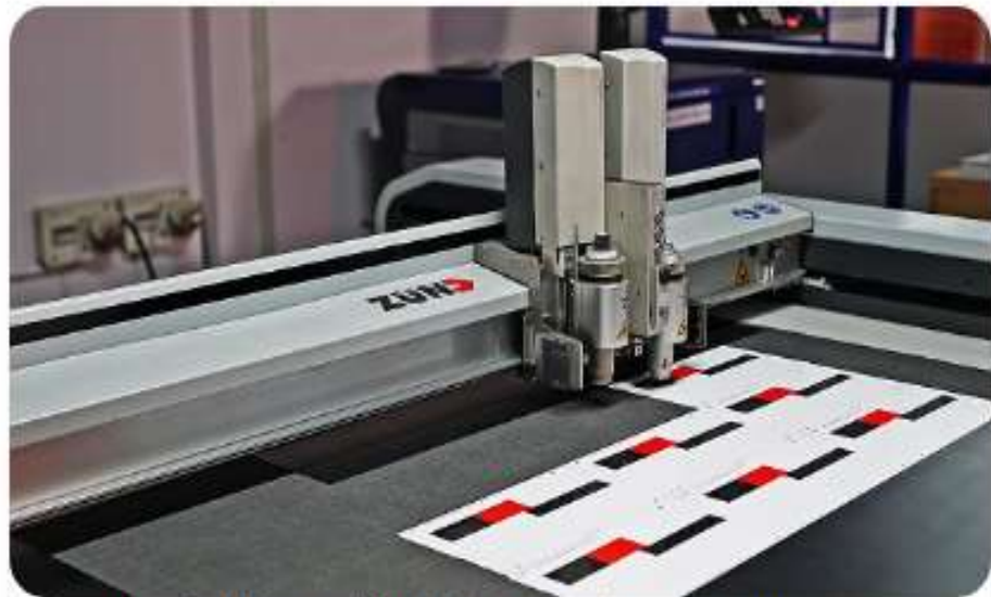
CNC cutting for high-precision label and overlay components
