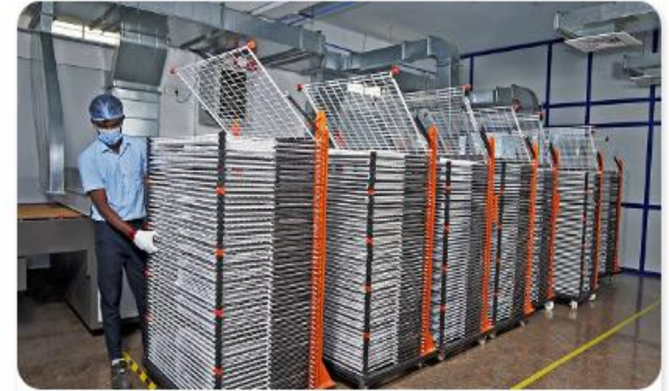
Batch-wise material handling and in-process storage system
