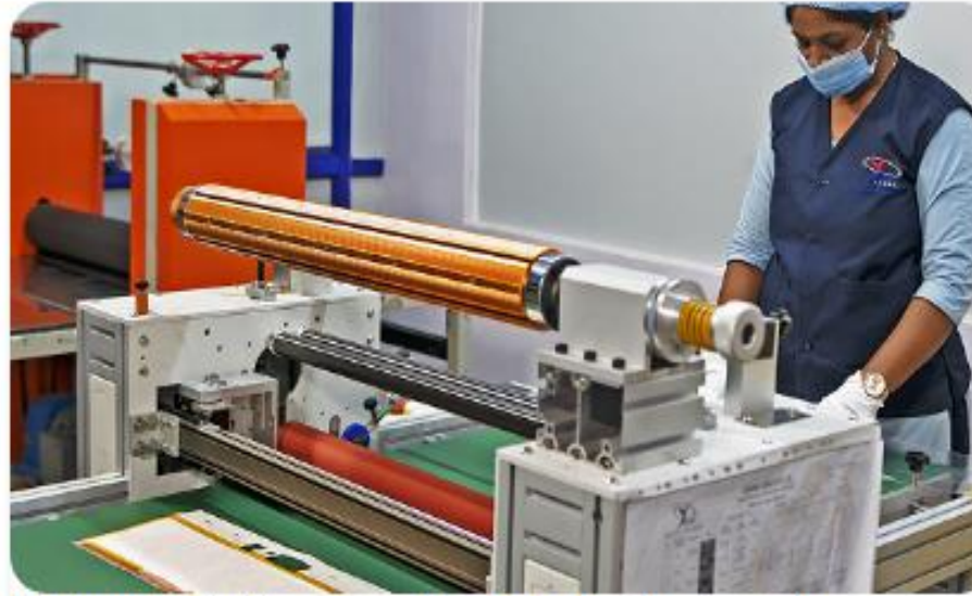
Roll-to-roll lamination process for label and overlay production
