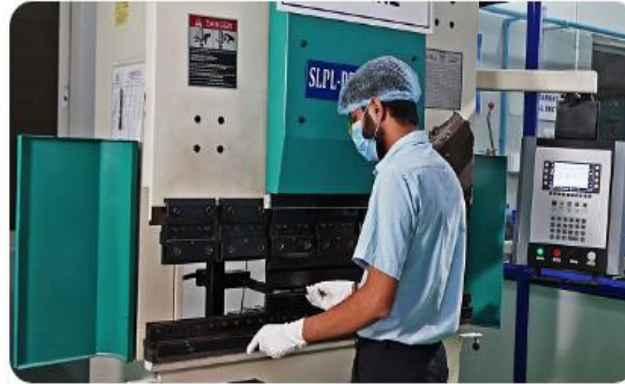
CNC bending machine for precision metal component fabrication
